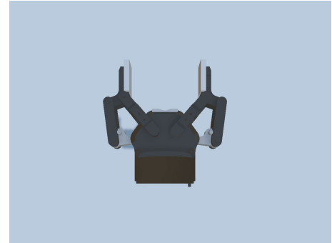
Sim Robotiq 2F-85 with constraint modeling
